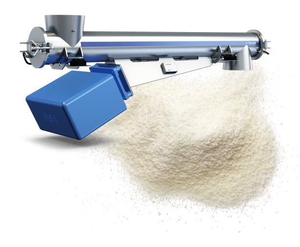
Tetra Pak® Vibrating Conveyor EV conveys and/or doses granulated or powder components over short distances. Connected to lean phase pneumatic transport via 88.9 mm diameter pipe of 50 or 80 metres. Electromagnetic motor. Manual operator control. Possible to vary vibrations from 0 to 70 Hz.
